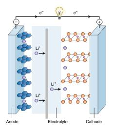
Fig. 1 | Components of a rechargeable Li-ion battery.
