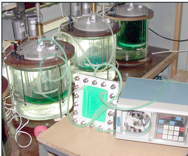
Setting for crystal growth including track nanomembrane cassette
