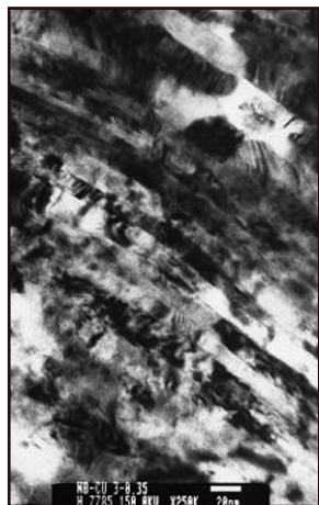
Structure of the nano-laminate Cu-Fe after cold rolling in the 3-rd cycle
